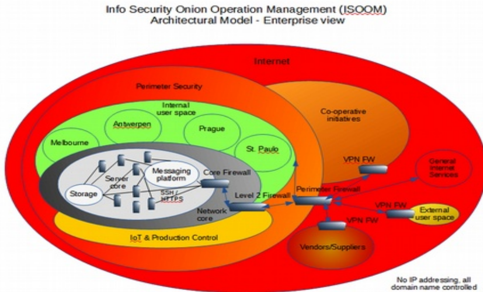
Figure 1: The ISOOM segregated network model
